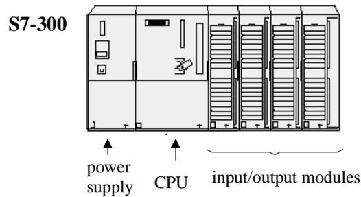
**Figure 2:** PLC with local input/output module.
