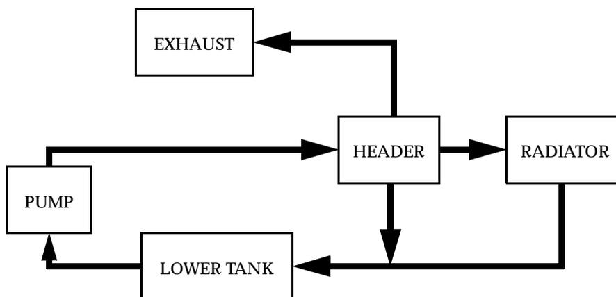
**Figure 10:** HMPID process architecture.
