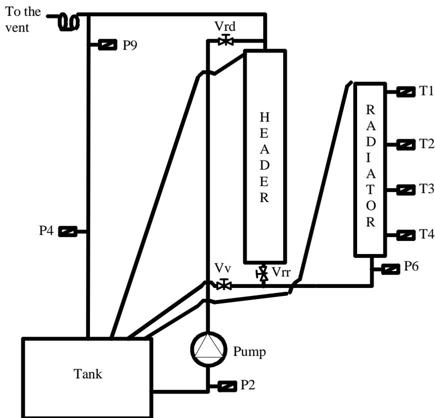
**Figure 1:** The HMPID C6F14 liquid distribution prototype.
