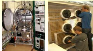
Fig. 7. CsI evaporation plant Fig. 8. Glove-box preparation.
