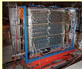
Fig. 13. Module 3 at the CERN/SPS-X5 test beam, fully equipped with the FEE and R/O electronics.
